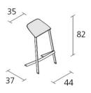
Stool with structure composed of extruded polished aluminium. Seat and back in plywood and expanded polyurethane, upholstered with Kvadrat® fabric.
